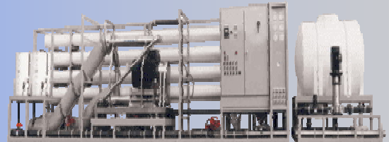
132,000 ~ GPD (500 M 3 /day) Seawater RO Plant with Energy Recovery Turbine
